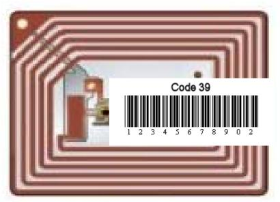
De RF transmitter/antenna detects and reads the chip containing Item IDentification
